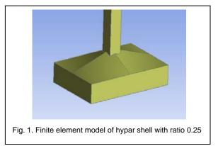
The dimensional details of hyper shell and rectangular footing are given in table 1 and 2. Dimension of edge beams and ridge beams are  $0.2 \text{ m} \times 0.5 \text{ m}$  and  $0.18 \text{ m} \times 0.4 \text{ m}$  respectively. For all the models same dimensions of edge and ridge beams are considered.
